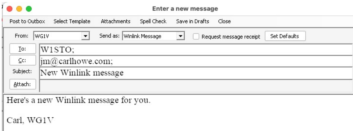
Figure 6: Winlink addresses can include Winlink user callsigns and standard email addresses separated by semicolons.
